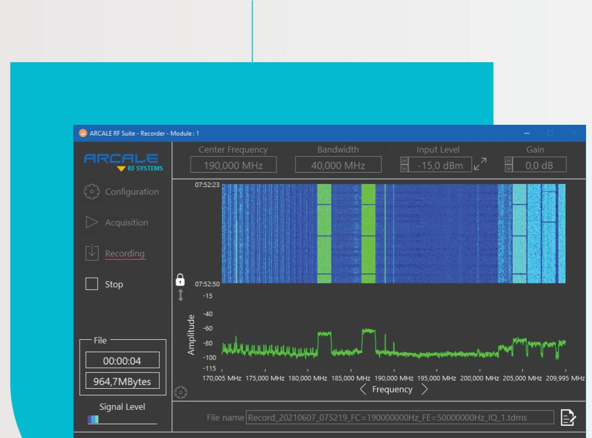
**ARCALE RF SUITE** is a modular software allowing various tasks on RF signals. Easy to configure and set-up, ARCALE RF Suite supports AirSpy, SignalHound, Tektronix, Harogic and National Instruments hardware.
